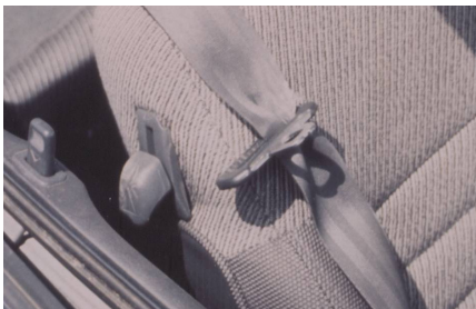
Examples of damaged webbing
