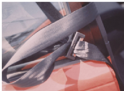
Examples of damaged webbing
